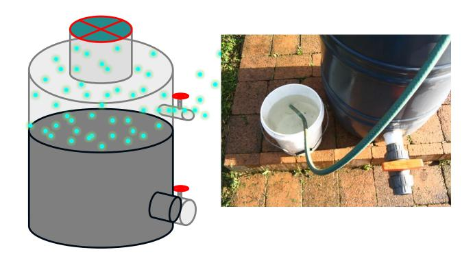
Alternatively attach a plastic hose to the ventilation valve and submerge the other end of the hose permanently in a bucket of water. Than open the valve. Any gas formed will naturally expel from the tank this way.
